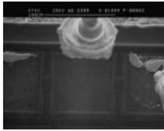
Picture 4. Typical bond failure with cavity tool. Bond sheared from bottom to top of picture. Ball diameter 70 \mu\text{m} .
