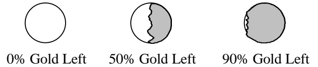
Figure 4. Sketch illustrating how a variable amount of gold is left on the pad after testing.
